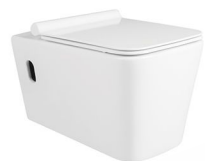
LJ-205 Wall hung toilet Size: 570x360x365 mm P-trap: 180 mm roughing-in
