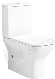
LJ-312 Two piece toilet Size: 620x360x800 mm S-trap: 250 mm roughing-in P-trap: 180 mm roughing-in
