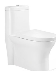
LJ-104 One piece toilet Size: 705x390x775 mm S-trap: 250/300 mm roughing-in
