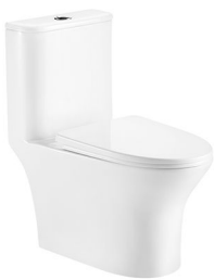
LJ-110 One piece toilet Size: 710x400x770 mm S-trap: 300 mm roughing-in
