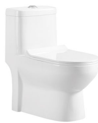
LJ-125 One piece toilet Size: 680x380x730 mm S-trap: 250/300 mm roughing-in P-trap: 180 mm roughing-in
