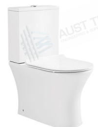
LJ-315 Two piece toilet Size: 615x360x805 mm S-trap: 250 mm roughing-in P-trap: 180 mm roughing-in
