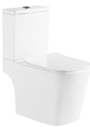
LJ-306 Two piece toilet Size: 650x365x785 mm S-trap: 250 mm roughing-in P-trap: 180 mm roughing-in
