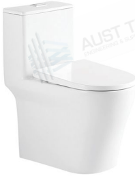
LJ-115 One piece toilet Size: 680x370x750 mm S-trap: 300 mm roughing-in
