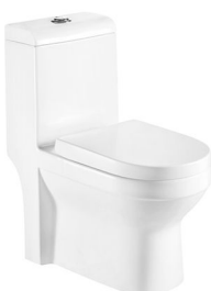
LJ-102 One piece toilet Size: 725x380x800 mm S-trap: 250/300 mm roughing-in P-trap: 180 mm roughing-in
