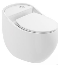
LJ-121 One piece toilet Size: 660x430x550 mm S-trap: 300 mm roughing-in
