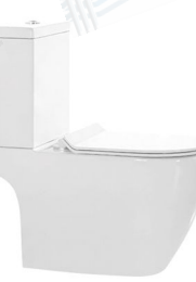
LJ-316 Two piece toilet Size: 660x365x800 mm S-trap: 250 mm roughing-in P-trap: 180 mm roughing-in
