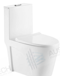
LJ-105 One piece toilet Size: 680x390x785 mm S-trap: 250/300 mm roughing-in P-trap: 180 mm roughing-in
