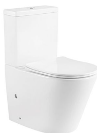
LJ-320 Two piece toilet Size: 605x370x800 mm S-trap: 100-250 mm roughing-in P-trap: 180 mm roughing-in
