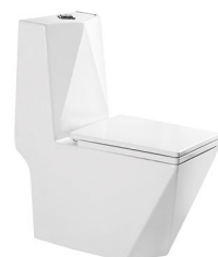
LJ-106 One piece toilet Size: 680x380x830 mm S-trap: 250/300 mm roughing-in P-trap: 180 mm roughing-in
