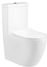
LJ-103 One piece toilet Size: 670x370x840 mm S-trap: 250 mm roughing-in P-trap: 180 mm roughing-in
